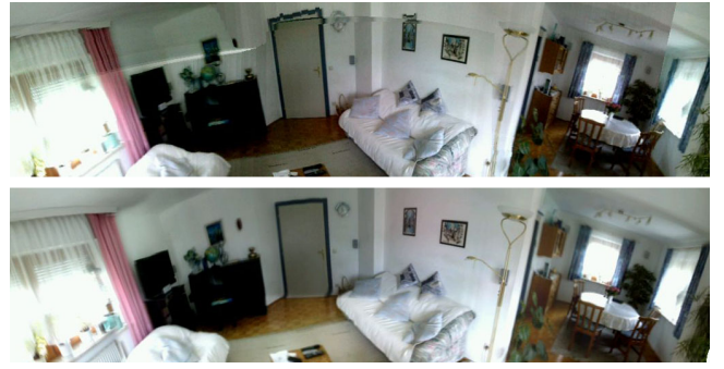
Figure 3: CPU-mapped image by the application of Wagner et al. [5] (above), GPU-mapped image with image refinements proposed (below).
