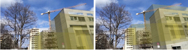
Fig. 6. Importance of IMU-to-camera calibration: (left) The building model is rendered with a proper calibration. (right) Through using an inaccurate calibration, the rotational error around all axes accumulates to about 6^\circ , which leads to a clear displacement of the virtual model from reality.
