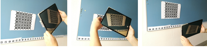
Fig. 5. Procedure to acquire calibration data: After assembling a rigid sensor setup, the user acquires the dataset. It is essential to perform a set of rotational and translational movements, as well as displacements of the sensors with respect to a calibration pattern in order to capture enough variation for the calibration method to perform properly.
