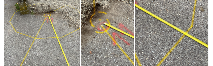
Fig. 12. Setup for our marking repeatability and accuracy test: (left) A tape measure is placed perpendicular to measure displacements of virtual spray marks. We measure (middle) the offset at the reference point and (right) the displacement at the 1m, 2m and 3m marking.
