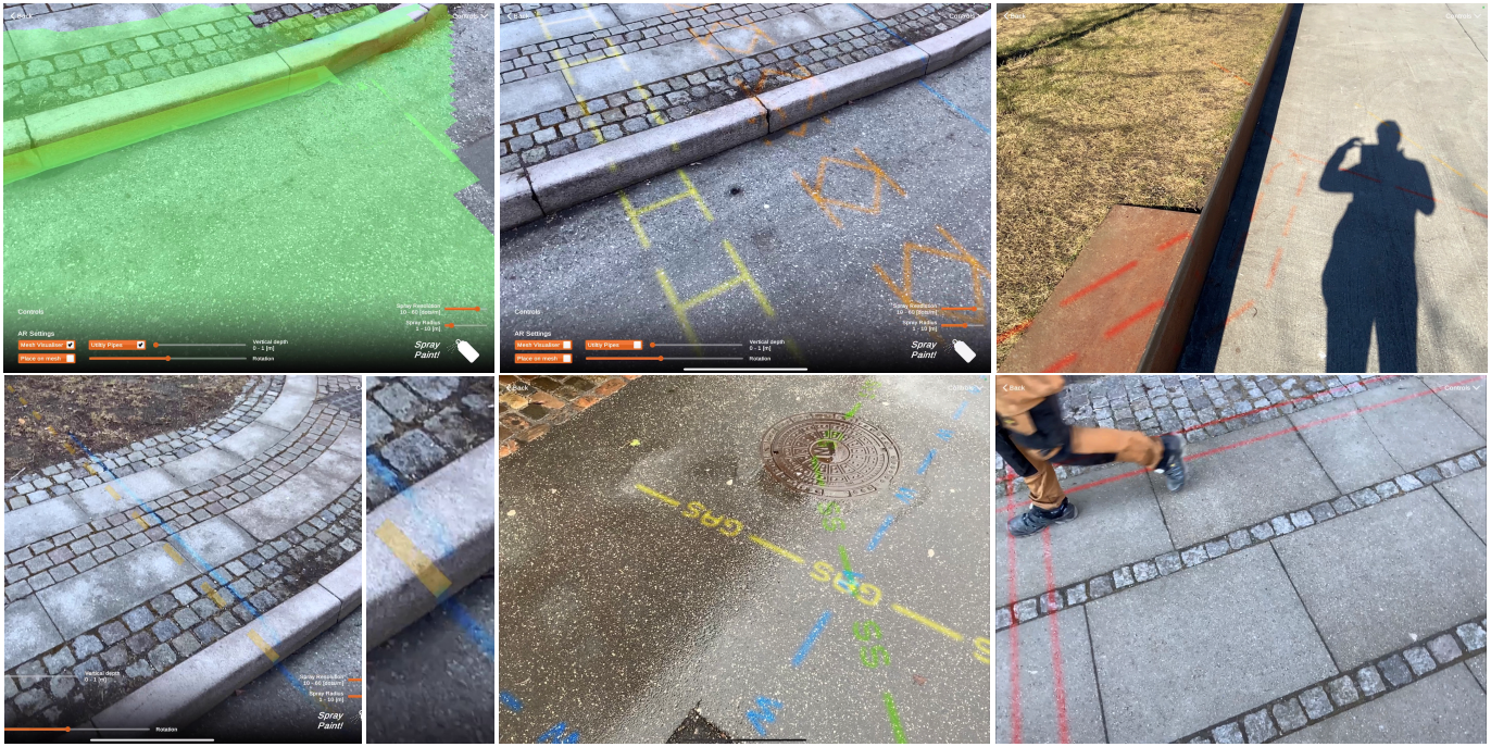
Fig. 14. Outdoor virtual utility marking using real GIS data: (top left) The mesh generation from LIDAR closely follows the real surface. (top mid) Virtual spray markings showing glyphs which respect the elevation change. (top right) Rendering with dynamic illumination. As the spray effect directly incorporates the shadows as seen by the camera, the spray markings fuse with reality in an indistinguishable way. (bottom left and inset) The orange dashed lines are showing the location of the subsurface utility as a naive overlay on the video, while the blue lines show the spray following the reconstructed surface. (bottom mid) Real subsurface utility data overlaid on wet surfaces. (bottom right) Using a feature to detect people, dynamic occlusion is correctly resolved.
