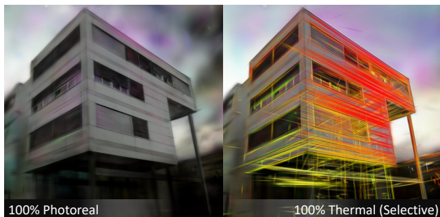
Figure 8: We apply a selector for the different modalities, as described in Figure 4 to achieve a selective visualization. Scene from the ThermoNeRF [11] dataset.
