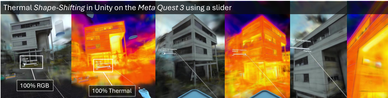
Figure 7: Thermal Shape-Shifting Splats: Three pairs of images with different viewpoints, resembling a user inspecting a building thermally while wearing the Meta Quest 3 . Each pair shows the extremes between purely RGB and purely thermal encodings. Using the slider, the user can choose between the modes (and any mixed mode in between), which are baked into the 3DGS model.
