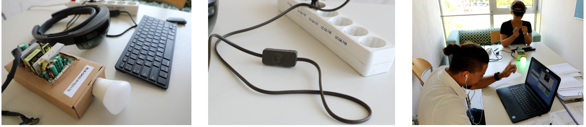
Figure 5: (left) User study equipment: faulty device (electronics box with light-bulb, with device id label on top, HoloLens and Bluetooth keyboard), (center) Power cord with labeled outlets Labeled outlets, (right) The worker wearing the HoloLens has completed the task, and the light-bulb turns green.
