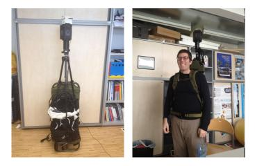
Fig. 2. Left: data acquisition system, consisting of the backpack, the *Point Grey Ladybug 3* camera mounted on a tripod and the antenna of the *Novatel* GPS receiver on top of the camera. Right: a user operating the acquisition system.
