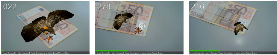
Fig. 8. Screenshots from the game taken on the mobile phone. The eagle is circling over the target, on which the system places animated prey. By placing prey it suggests a new viewing position the user should reach with the mobile device to make the eagle attack and score.
