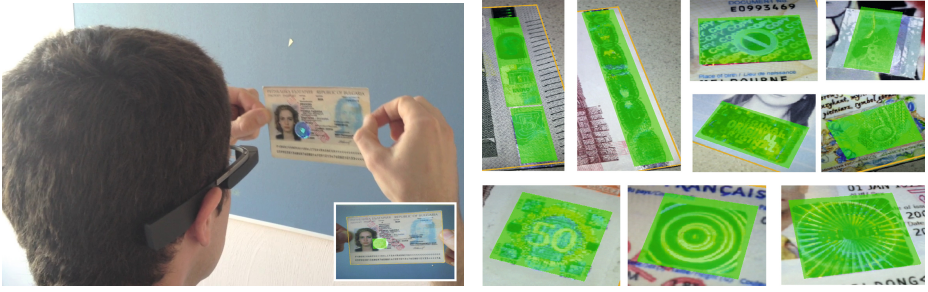
Fig. 4. Left: Using Google Glass to perform hologram detection on a foreign passport. Right: Augmented detection results of exemplary samples using in our evaluation.
