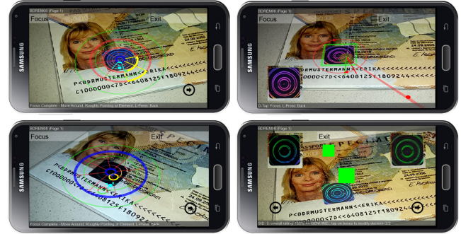
Figure 1: User interfaces for hologram verification: Constrained navigation (top-left), alignment (top-right) and hybrid user interfaces (bottom-left) are designed, implemented and evaluated within a user study. They allow to reliably capture image data suitable for automatic verification. Results are presented to the user in a summary (bottom-right).
