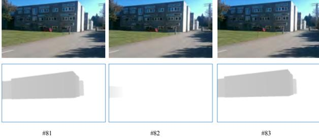
Figure 3: The drift problem of GPS sensors. Top: Three images from dataset 07-08. Bottom: Corresponding depth images calculated from the raw sensor pose. While the first and the last frame have reasonable pose estimates, the pose of the middle frame suffers from a completely wrong estimate due to temporal GPS drift.
