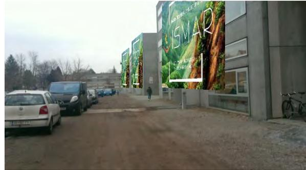
Figure 1: Results from our SLAM-based localization system after optimization. Left: an overlay of the 2.5D building model from OpenStreetMap. Right: ISMAR logos superimposed onto the façades using the surfaces from the 2.5D maps.
