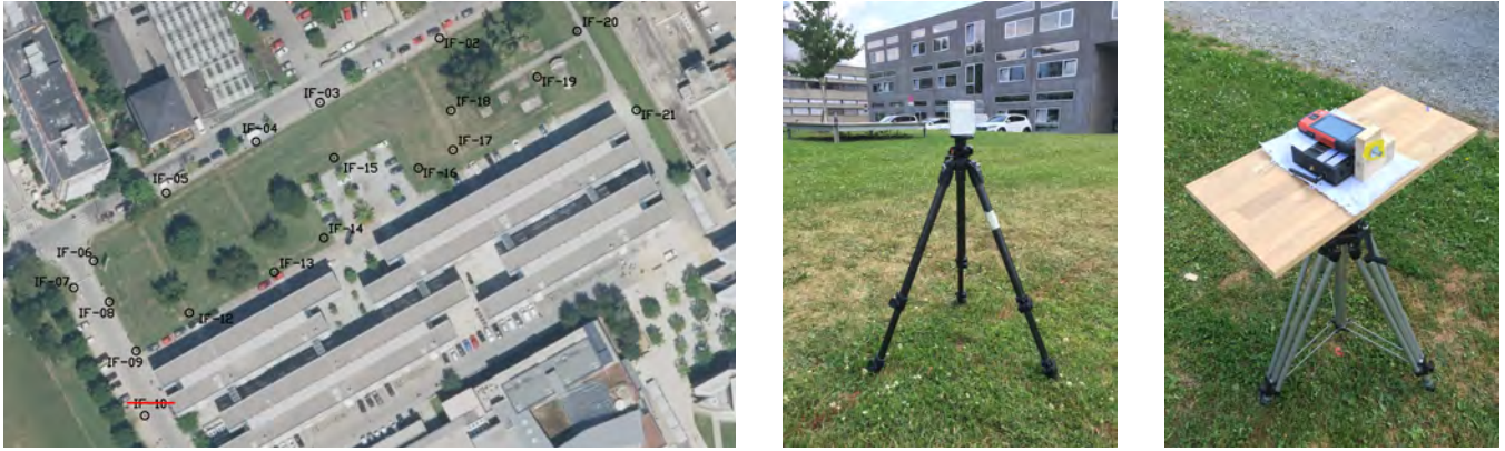
Figure 4: Environment setup for the compass validation. Left: Map of all reference Points. Middle: Reflective prism on a tripod. Right: Laser range finder mounted on the sensor cube.
