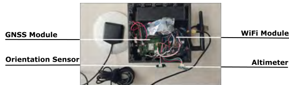
Figure 1: Left: First prototype of the sensor cube labeled with its components. Middle, right: GIS data Visualization of buildings at the university using Unity.
