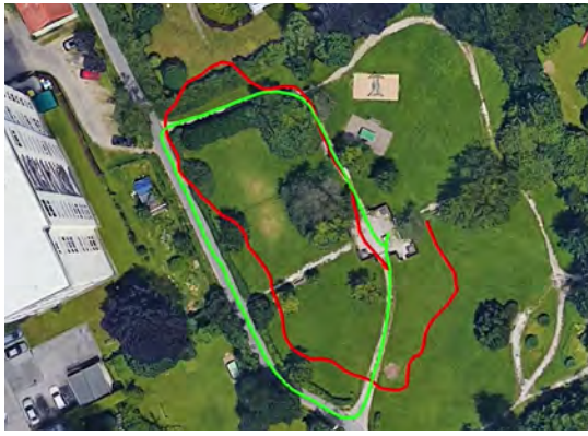
Figure 3: GPS track of a walk through the park, comparing mobile built-in GPS to the uBlox receiver. Green: uBlox Red: LG G5
