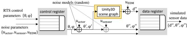
Fig. 4. Sensor hardware uncertainty model of the RTS simulator. The noise parameters can be controlled externally which allows simulation of different hardware specifications and measurement setups;  $u_{actuator}$  and  $u_{sensor}$  are the actuator and sensor uncertainties respectively;  $u_{EDM}$  is the distance measurement uncertainty.
