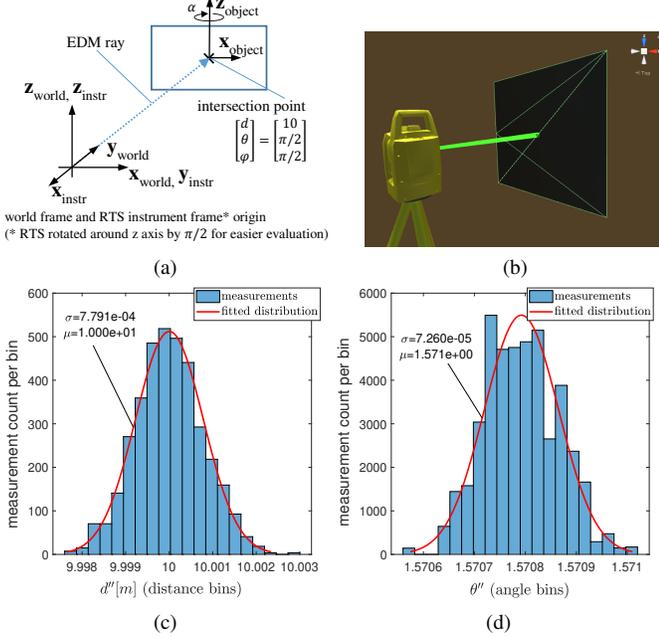
Fig. 5. Sensor hardware noise simulations. (a) Uncertainty verification concept. (b) Unity3D setup for simulation uncertainty verification. (c) EDM noise:  $u_1(x') = 0.75 \times 10^{-3} \text{m}$ ,  $u_2(x') = 10 \times 10^{-6}$ . (d) angle sensor noise:  $u_1(x') = 5'' \approx 24.241 \times 10^{-6} \text{rad}$ ,  $u_2(x') = 0$ .
