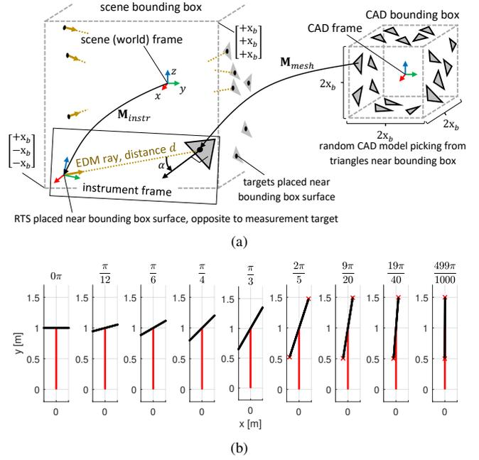
Fig. 9. Setup of MC uncertainty experiments for analyzing influences of floating-point arithmetic. (a) object frames and transformations. (b) Varying incident angle experiments (top view, EDM ray and measured plane, instrument frame).
