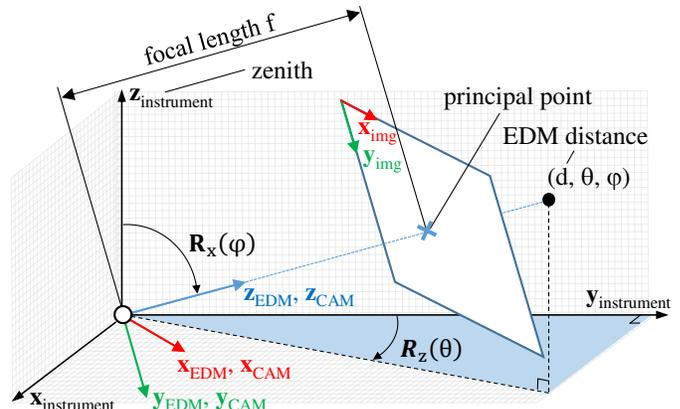
Fig. 1. Simple geometric model of an RTS with a camera module, as used by Klug *et al.* [5].
