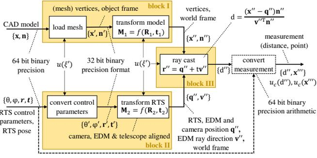
Fig. 7. Uncertainty propagation in the simulator pipeline, partitioned into three processing blocks.
