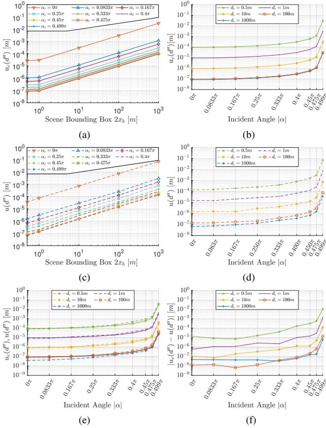
Fig. 10. Uncertainty estimations of EDM intersection points for the RTS simulator. Analytical uncertainty: with respect to the scene bounding box (a), with respect to the incident angle (b). Uncertainty using MC experiments: with respect to the measured scene bounding box (c), with respect to the incident angle (d). Analytical uncertainty  $u_c(d'')$  (continuous lines) compared with MC experiments (dashed lines), plotted with respect to the incident angle (e,f).
