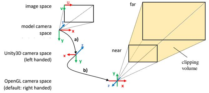
Fig. 3. Transformation between RTS model, Unity3D and OpenGL: a) convert camera space RTS model to Unity3D, b) convert camera space from Unity3D to OpenGL.
