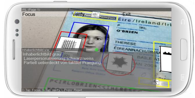
Fig. 3. Mobile document verification system tracking a sample instance of the data page used in passport. The position of security features is augmented directly onto the document. Detailed information about an element can be triggered by pointing the camera at it.
