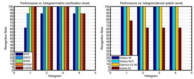
Fig. 6. Left: Performance in recognizing fake and original holograms by majority voting on patch matching results under various office conditions. Right: Performance in recognizing fake and original patches when using various devices under optimal office conditions.
