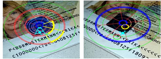
Fig. 8. AR UIs with guidance for interesting subspaces. Either pie-slices (left) or circular regions (right) can be indicated for sampling. In the first case, this corresponds to a constrained navigation space, while in the second case final alignment with the circular regions is required (hybrid).
