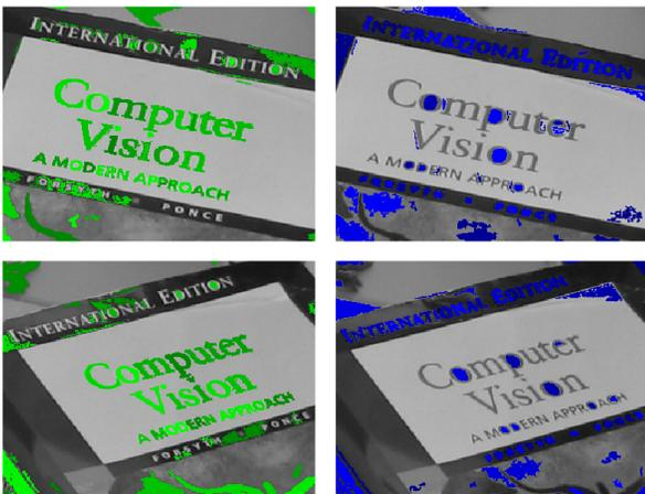
Figure 5. Image tiles cropped with overlaid MSER detection results for positive regions and negative regions on the left, respectively right side. The images are separated by an approximately 30° viewpoint change. As can easily be seen the regions found by the algorithm are almost the same for both views.
