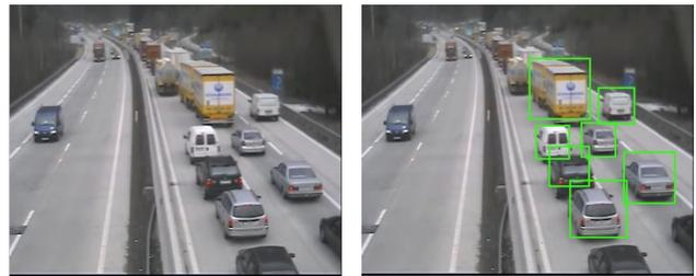
Figure 4. A frame taken from a different video stream and the results of both algorithms. The simple system simply fails because objects are “fading” into the background model (left). The upgraded system can still detect all objects correctly because the algorithm simply scans over the whole image if no region of interest has been found by the previous module.
