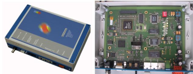
Figure 1. Prototype of the embedded DSP vision platform.
