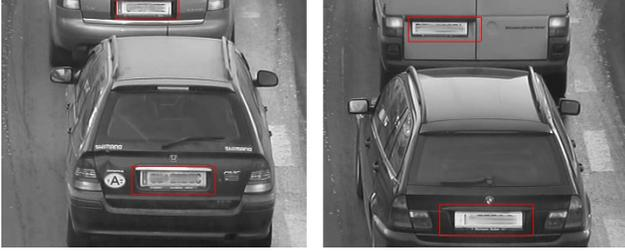
Figure 6. Two frames taken from a 15 minutes demonstration video and the results our algorithm. Note, that the region inside the bounding box should now be passed to an OCR module for further processing.
