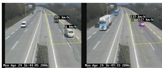
Figure 5. Two frames taken from a 30 minutes demonstration video and the results of our algorithm. As can easily be seen, in both frames, both vehicles were successfully tracked. The corners of the yellow rectangle represent the four reference points used for homography calculation.
