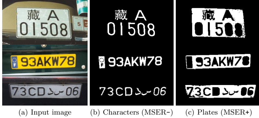
Fig. 3. Detection results on international license plates where (b) shows the segmented signs detected as MSER- and (c) the plate detected as MSER+. As can be seen the detection algorithm can be applied to any international type, because the criterion used in the detection algorithm is valid for all cases.
