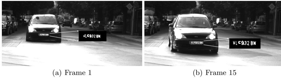
Fig. 4. Illustration of license plate tracking. The images show a traffic scene and the segmented characters on the license plate are highlighted in white.
