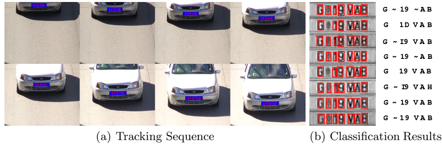
Fig. 5. Recognition is improved by using several license plate representations provided by the tracking scheme. The final result based on a majority voting for this plate sequence is G~19VAB which matches with the real plate number.
