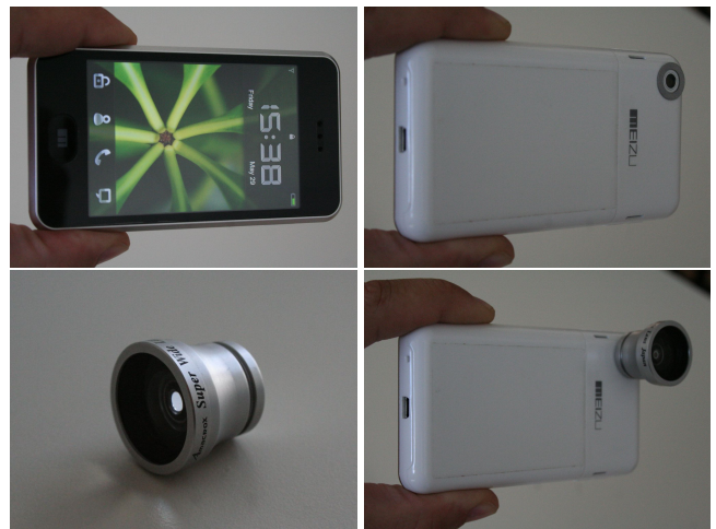
Figure 7: Meizu M8 mobile phone front view, back view with magnetic mounting ring, wide angle camera lens from AmacroX , mounted camera lens (from upper left to lower right).
