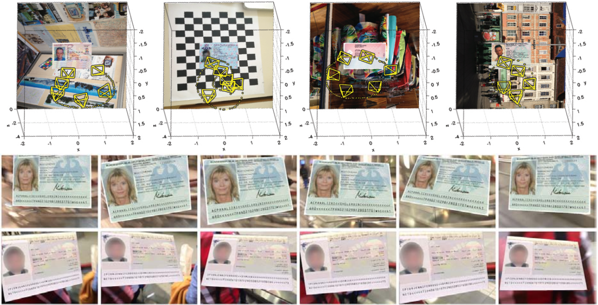
Figure 8: Top: Sequences of frames rendered onto a random background, and the corresponding camera trajectory. For better visibility, only every 25 th frame is drawn as a frustum. Bottom: Sample frames from two sequences. As the document is rendered into a video, the background changes with each frame.
